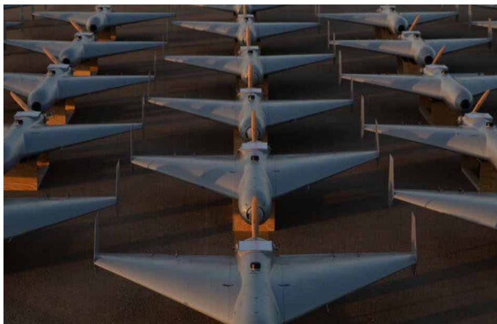
The Low-cost Unmanned Combat Attack System, or LUCAS, drones can be built at a small fraction of the price of earlier drones and are modeled after Iranian drones. U.S. Central Command
